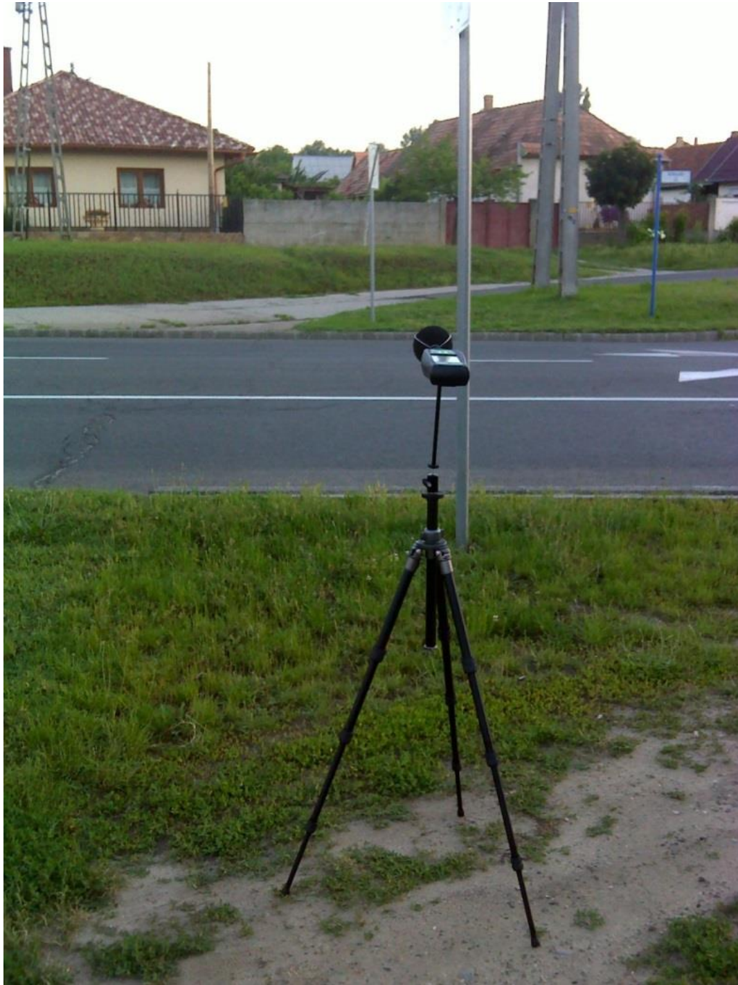
Figure 2-7: The position of the measurement microphone at measurement point No ZMP13 during the assessment of the ambient noise benchline level.
