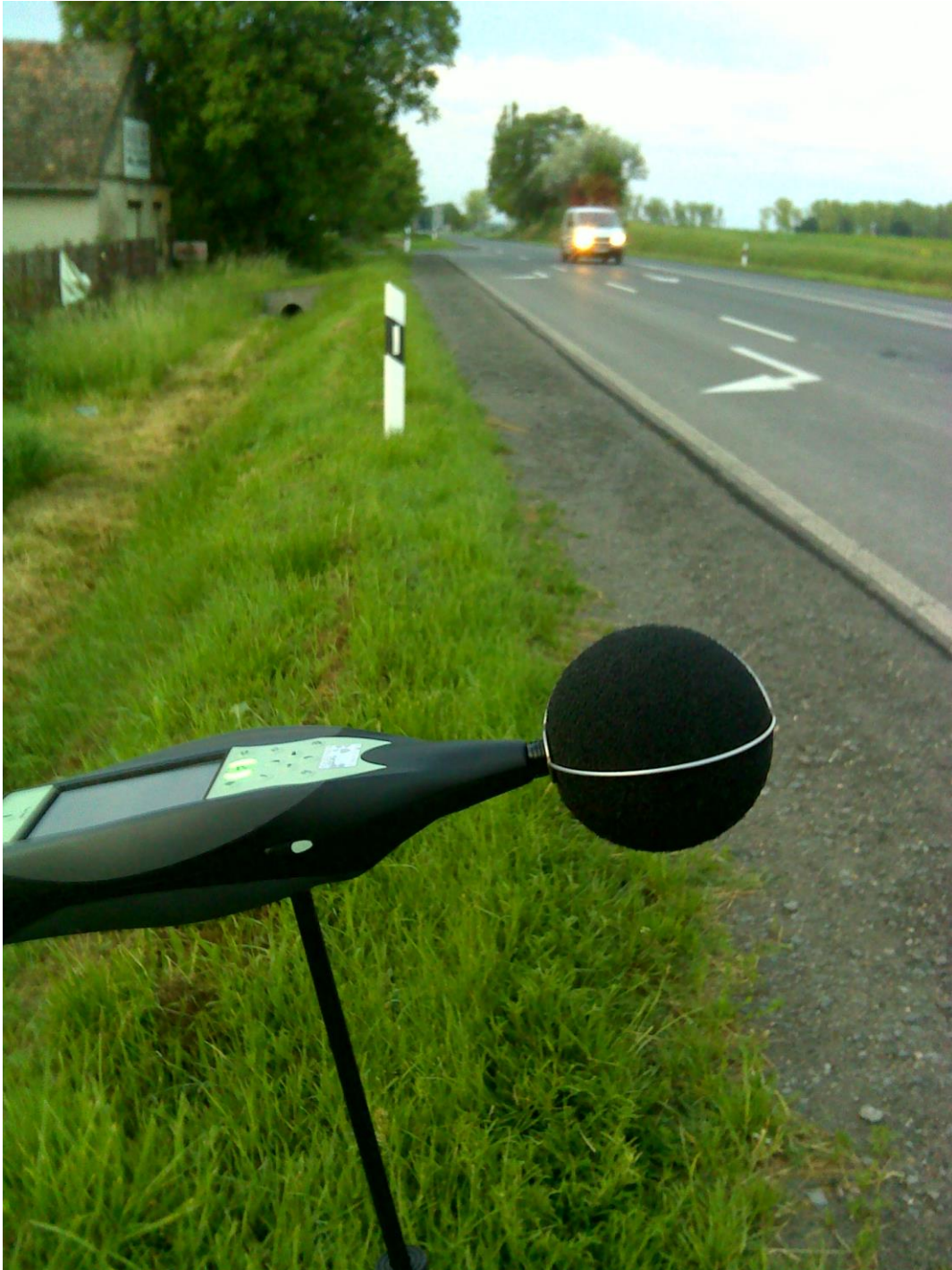
Figure 2-5: The position of the measurement microphone at measurement point No ZMP14 during the assessment of the ambient noise benchline level.
