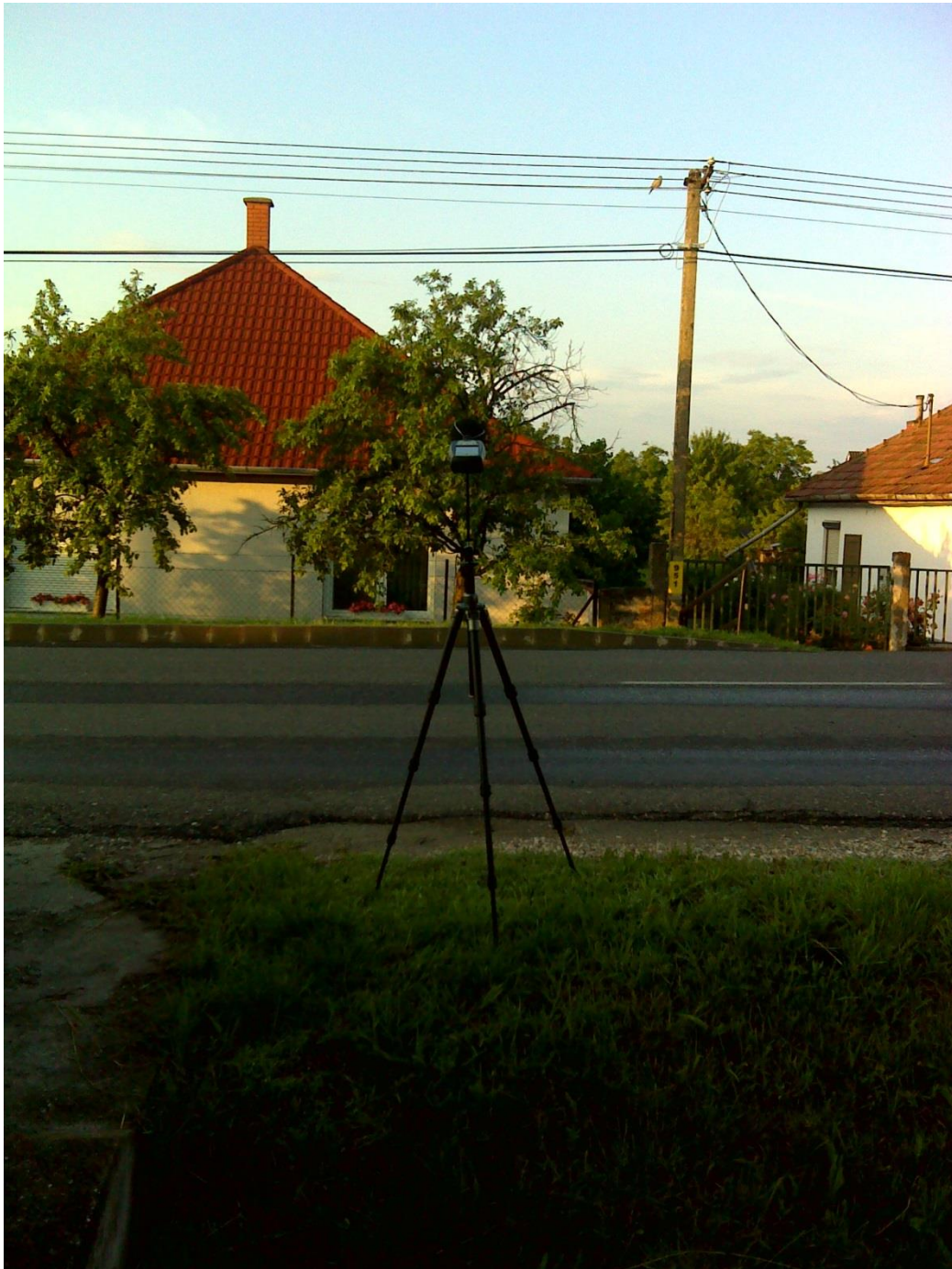
Figure 2-6: The position of the measurement microphone at measurement point No ZMP12 during the assessment of the ambient noise benchline level.
