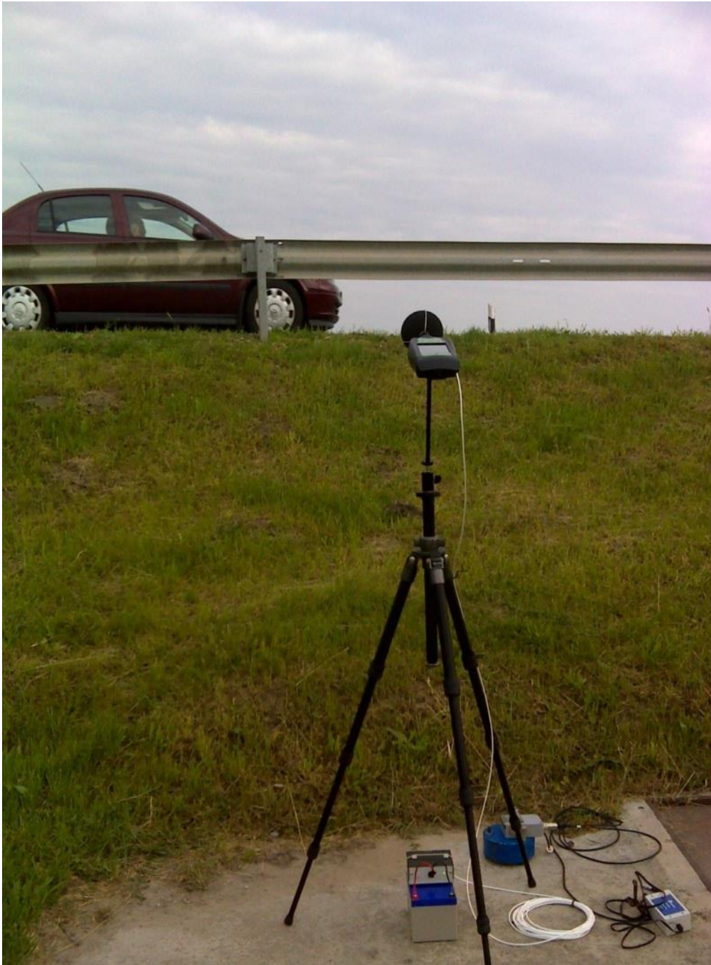
Figure 2-3: The position of the measurement microphone at measurement point No ZMP9 during the assessment of the ambient noise benchline level.
