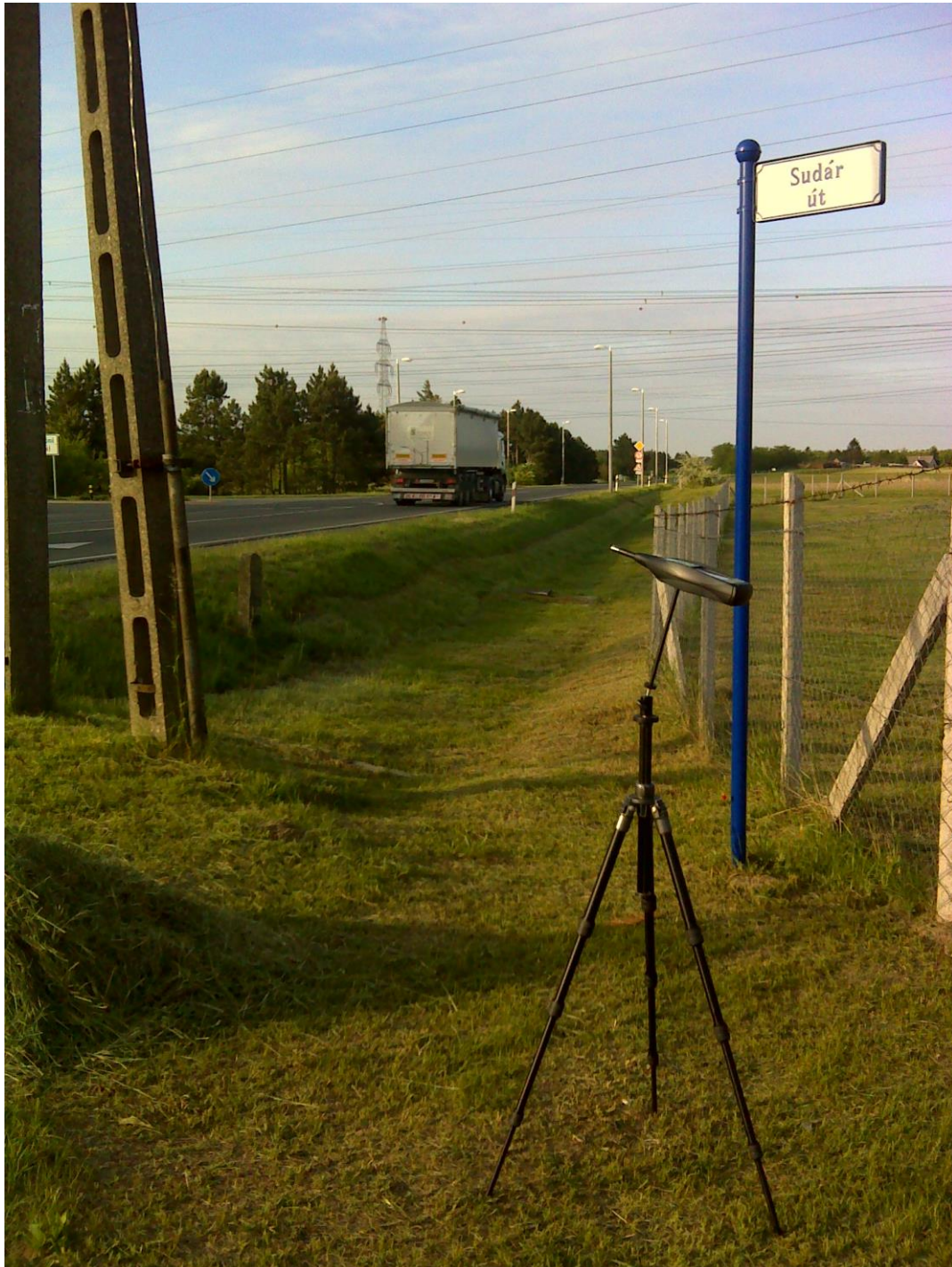
Figure 2-4: The position of the measurement microphone at measurement point No ZMP5 during the assessment of the ambient noise benchline level.
