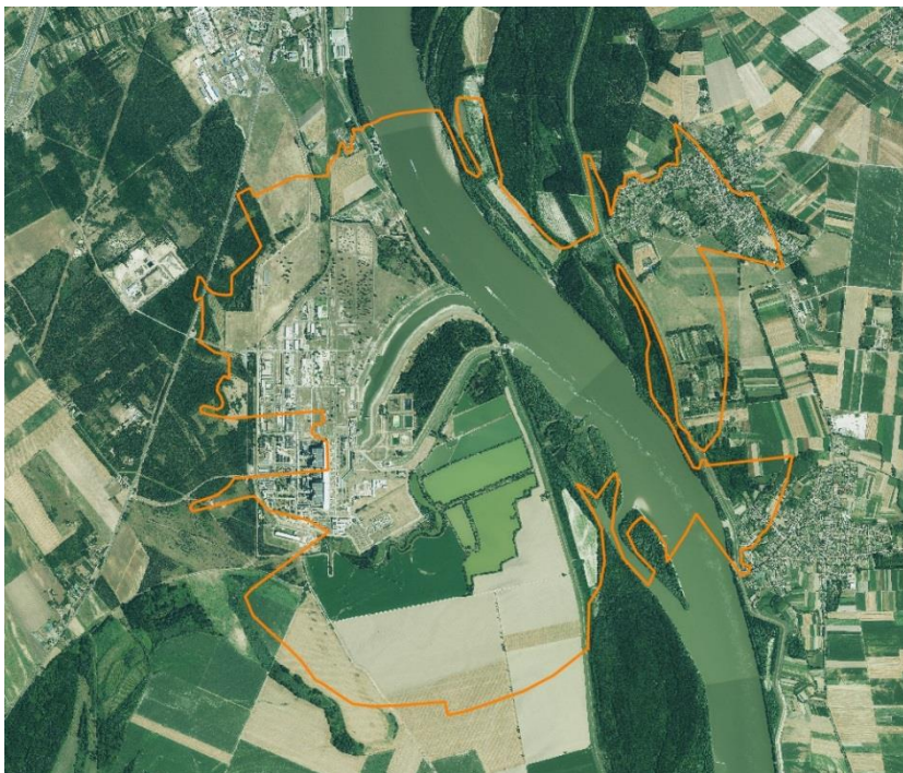
Figure 3.4-8: Noise exposure impact area of joint operation of Paks II. and Paks Nuclear Power Plant combined with the operation of transmission lines
